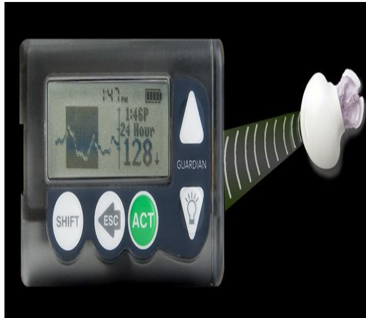
Figure 2: Guardian REAL-Time (Medtronic) for continuous glucose monitoring.
