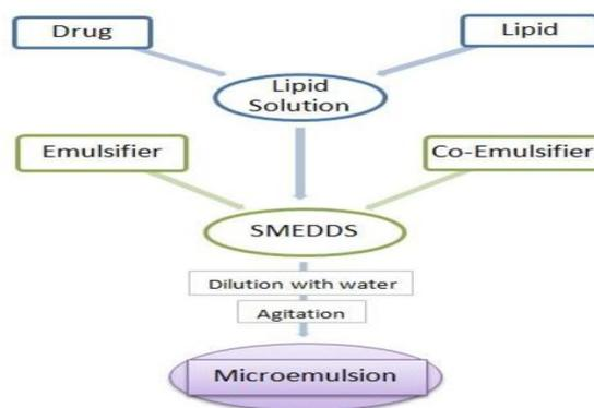
Fig. 3 General procedure for preparation of microemulsion
